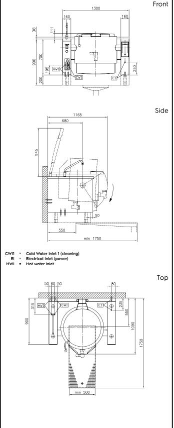
ProThermetic Sprint Electric Tilting Boiling Pan, 150lt Hygienic Profile, Freestanding with Stirrer and Variable Speed The company reserves the right to make modifications to the products without prior notice. All information correct at time of printing.
